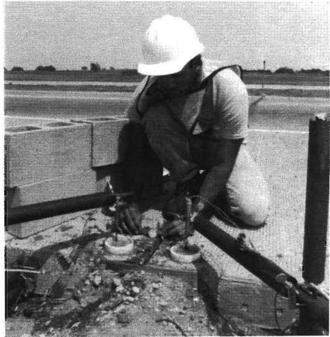
Fig 3.8. Joint width measurement using dial-caliper.
