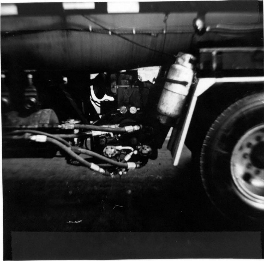
Side view of Deutz asphalt pump on distributor.
