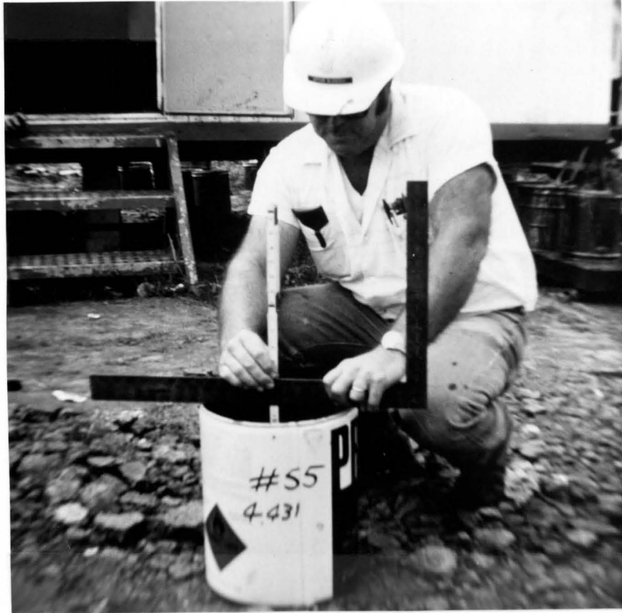
Calibrated bucket used to determine weight per gallon of each distributor load of asphalt rubber mixture.
