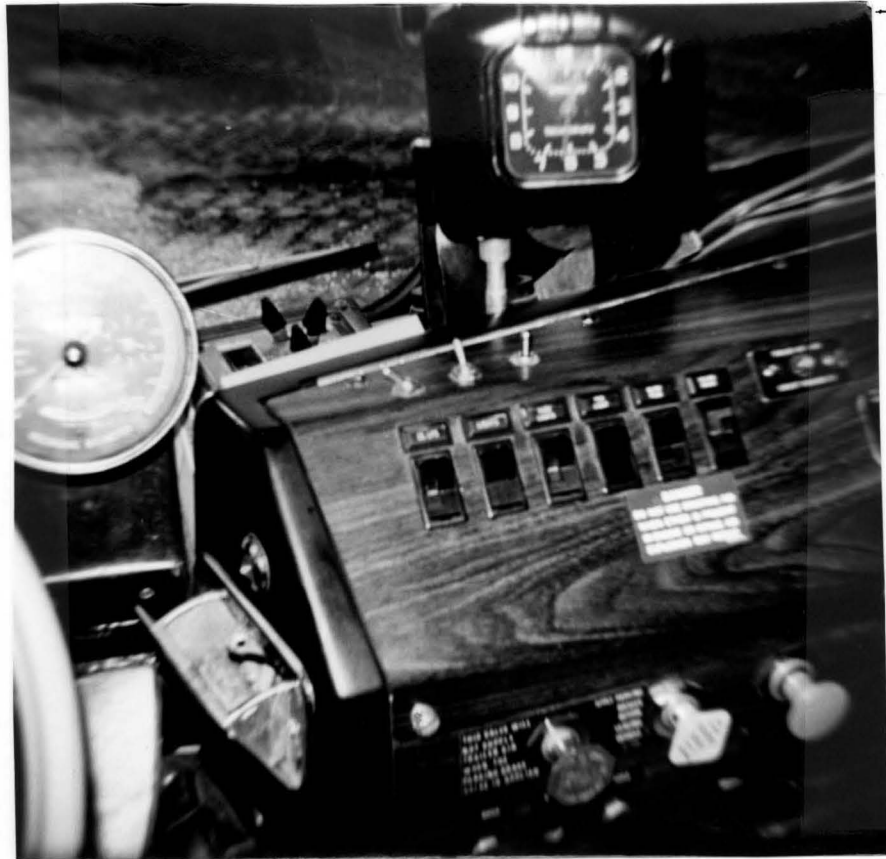
Instruments inside cab of distributor. Shows tachometer, speedometer, etc.
