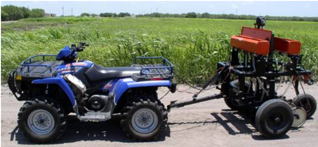
Figure 3-11. USDA, NRCS, “Kika” de la Garza Plant Materials Center ATV seed drill.
