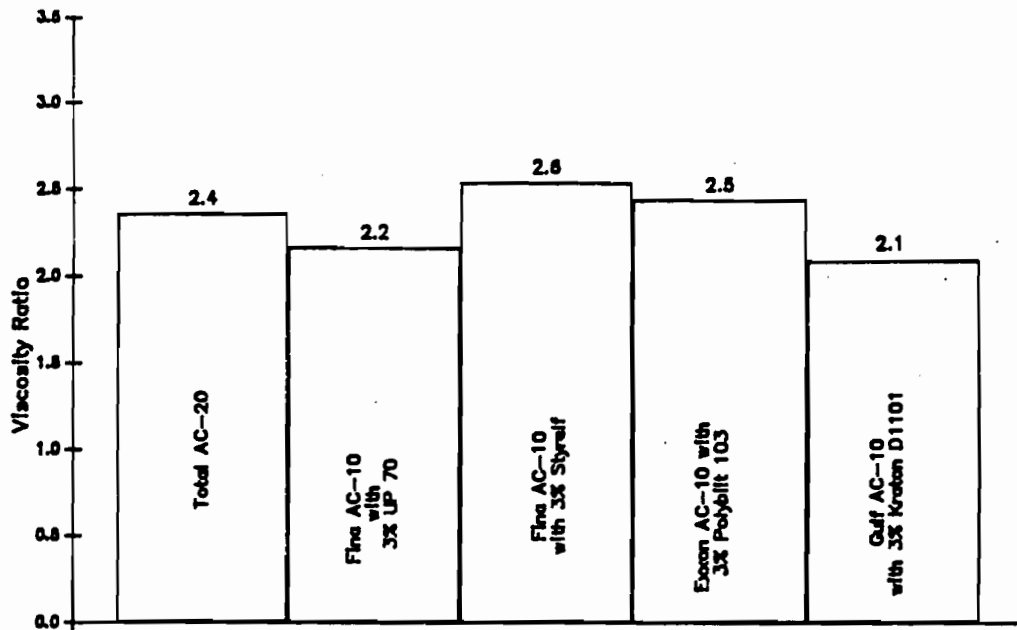
Fig. D-7 Viscosity Ratio at 140F for Unmodified and Modified Binders. (District 10)
