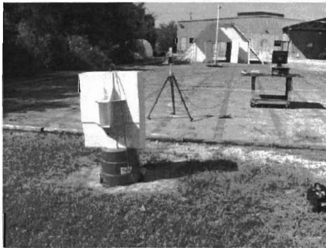
Figure 18 set up for the air-coupled GPR wireless radiation testing
