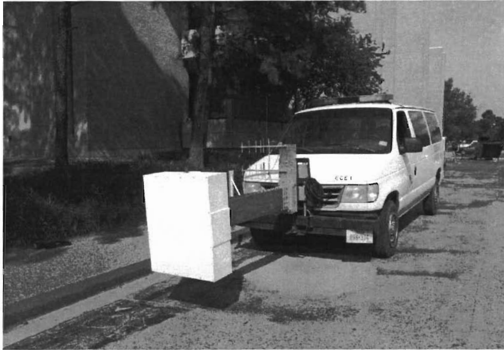
Figure 14 Air-coupled GPR mounted on a vehicle in application
