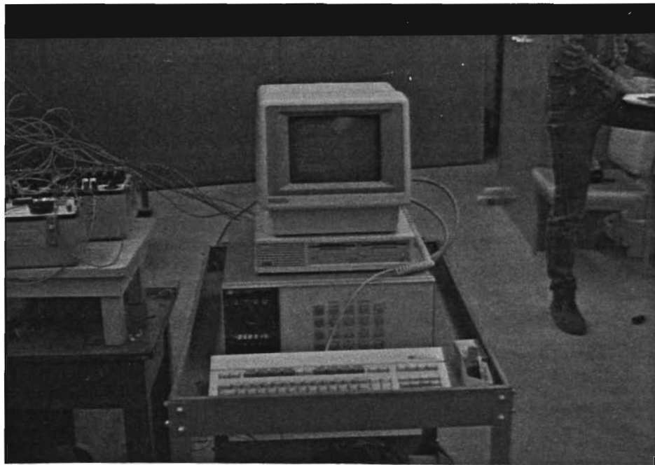
Fig 5.28. Strain and temperature monitoring devices used during thermal expansion experimentation.
