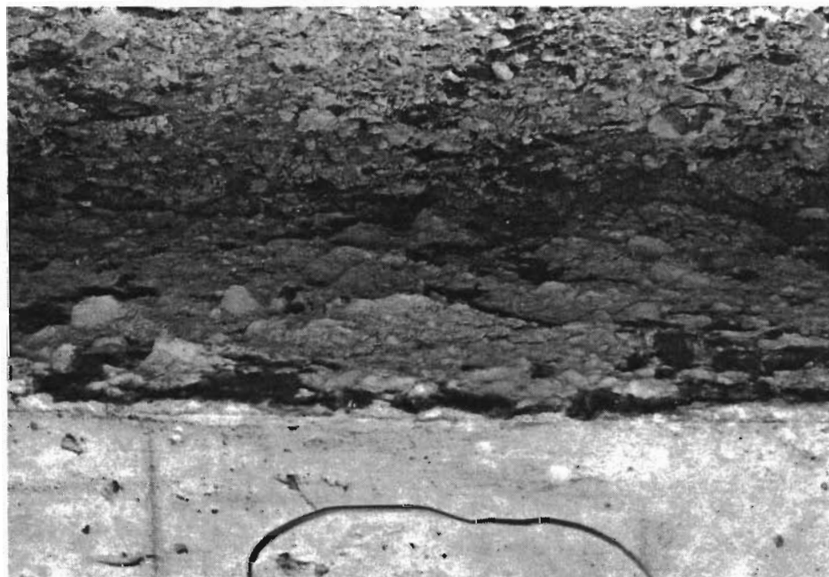
Fig 6.6. Observation of failure plane after push-off test on 4-inch slab over a flexible subbase. (continued)
