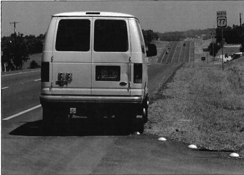
Figure 26. Dynatest Consulting Inc. Preparing to Collect Inertial Profile Data on US 77 in Waco.
