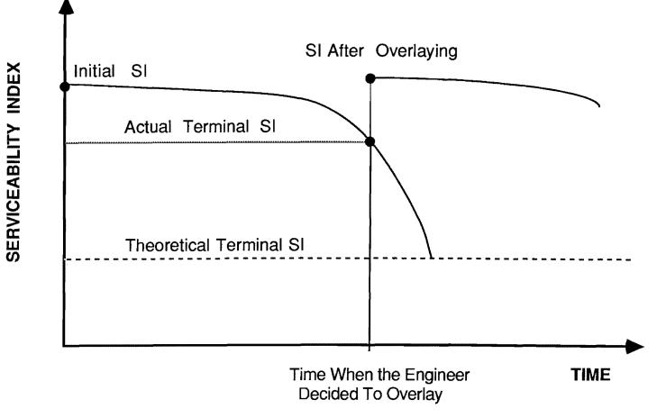
Fig 6.1. Location of the serviceability indices on the performance curve of a rigid pavement.
