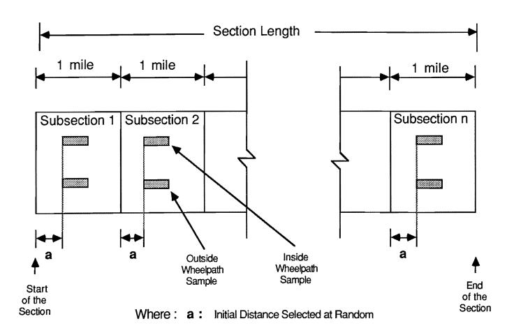
Fig 4.4. Sampling technique used within a section.
