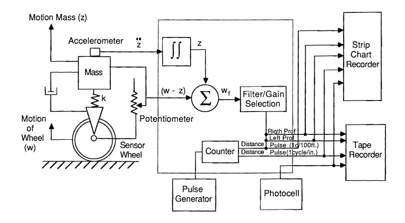
Fig 3.1. Schematic diagram of the SDP measurement system (after Ref 21).
