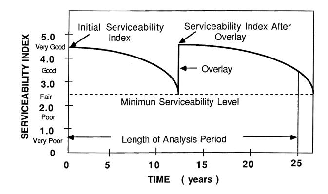
Fig 2.2. Example of a performance curve for one pavement design strategy (after Ref 3).
