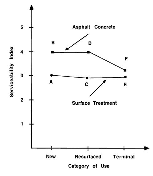
Fig 5.6. Surface type and category of use SI-interaction-flexible pavements.
