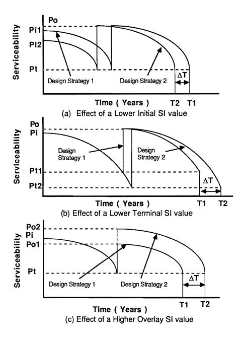
Fig 2.3. Effect of the design SI values on pavement performance.
