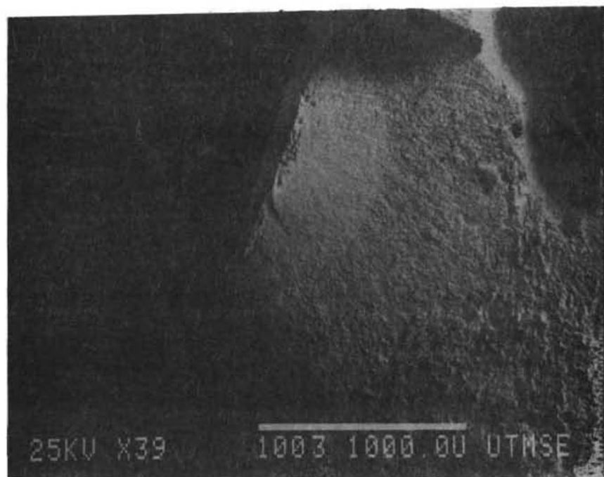
Fig. 6.9 Crack propagation plane
