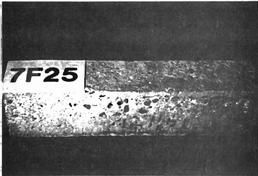
Fig. 5.27 Seven sack mix specimen subjected to 300 freeze-thaw cycles containing 25% Type A fly ash.
