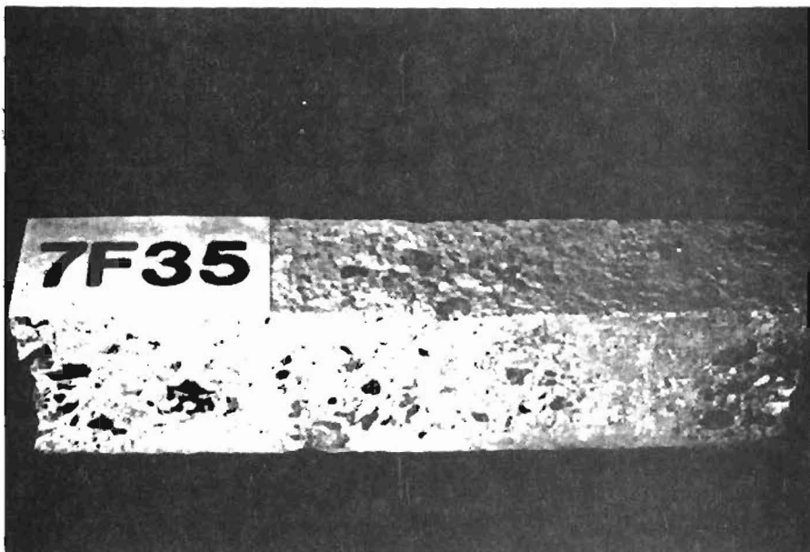
Fig. 5.28 Seven sack mix specimen subjected to 300 freeze-thaw cycles containing 35% Type A fly ash.
