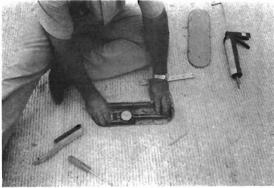
Fig 3. 9. Typical concrete movement measurement on inside plugs. Note easy access and position of hands. Also note standard bar on BCO surface.
