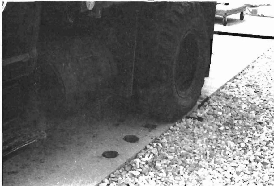
Fig 3.10. Static loading by means of a single axle dual tire truck.
