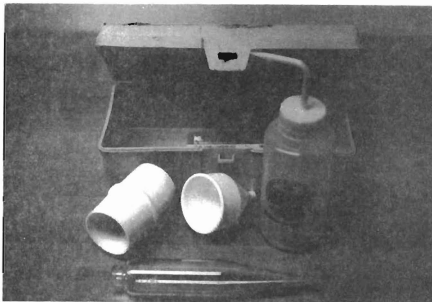
Fig. 2.3. Equipment for sand-content test.
