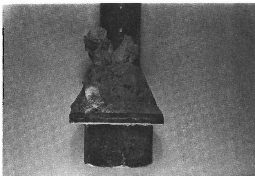
Fig. 4.17 Anchor bolts after removal from test specimen showing cone of compacted concrete
