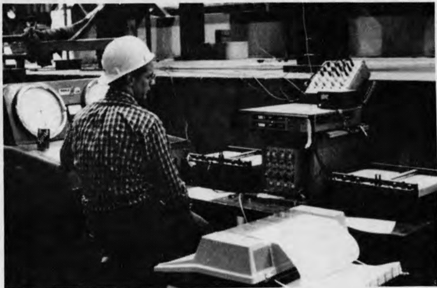
Fig. 3.33 Test setup; pulsator pump and pressure gages, plotters, power supply, peak detector, and computer terminal
