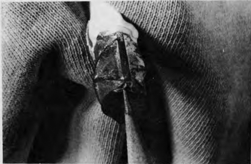
Fig. 3.44 Oval surface at a fatigue initiation crack
