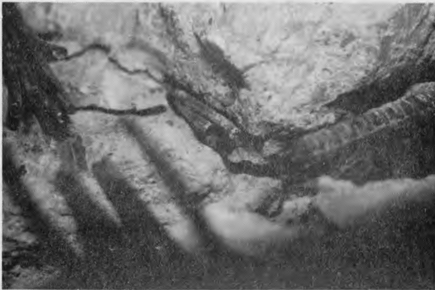
Fig. 3.40 Static wire break with necking
