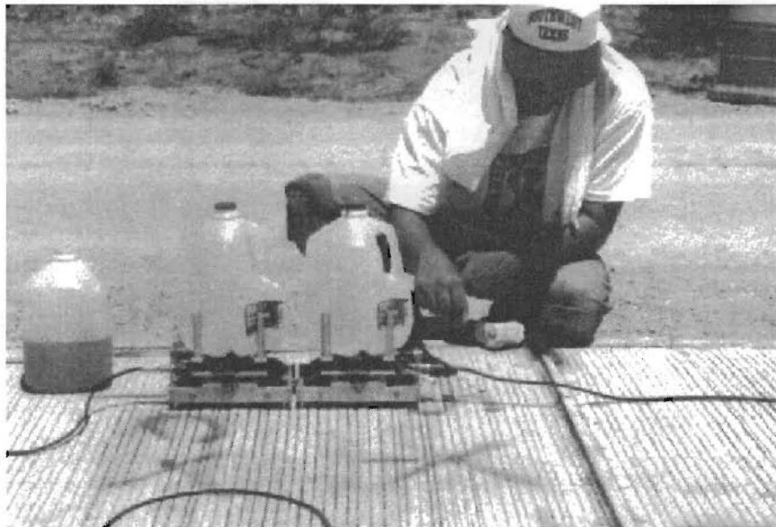
Figure 4.13 Impact-echo testing using equipment supplied by Olson Engineering
