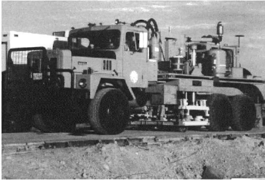
Figure 4.11 Rolling Dynamic Deflectometer (RDD)
