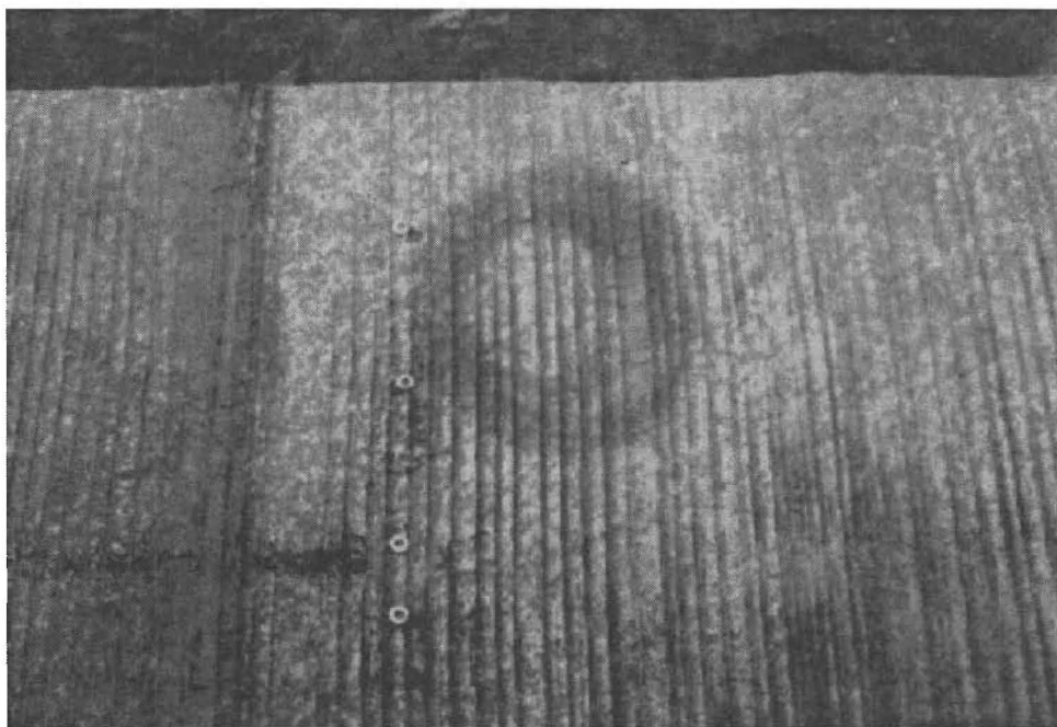
Figure 6.19 Steel washers used to attach magnetic accelerometers
