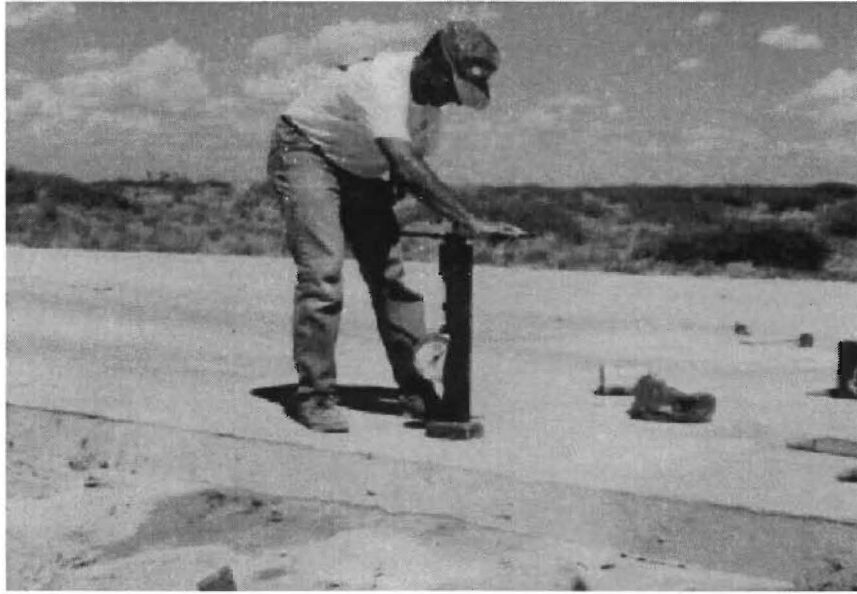
Figure 4.9 Pull-off testing procedure
