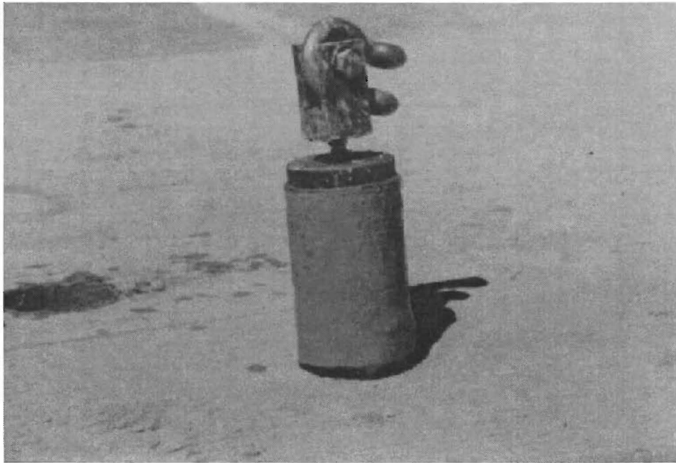
Figure 6.2 Pull-off test specimen after bond failure
