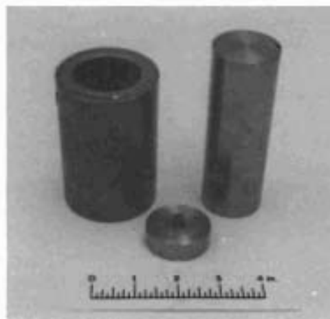
(a) Compaction mold, base plate, and ram, from left to right.
