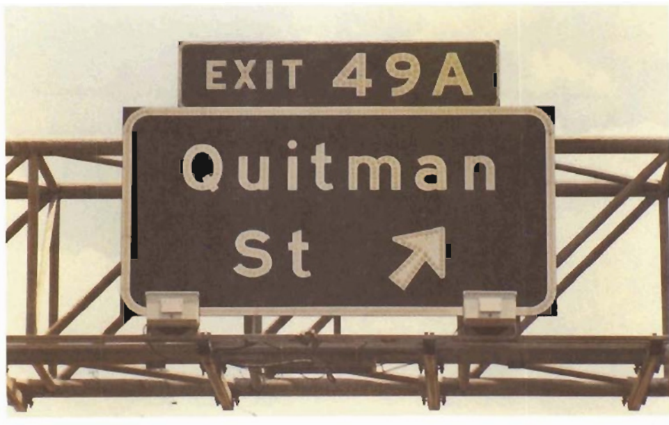
GES - 2C Green Sign Paint without Topcoat - 8 Years Field Service Good Condition in regards to color and surface condition
