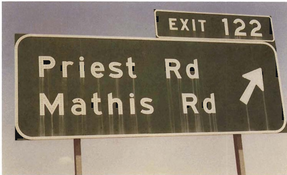
Figure 9: Thermal Setting Polyester Coated Legend chalking and running down Engineer Grade Reflective Sheeting Background Sign in San Antonio.
