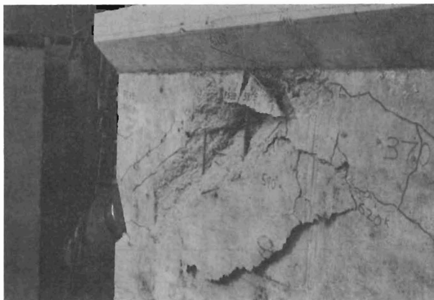
(a) Ultimate load: 590 kips. Side face rupture at point of maximum curvature
