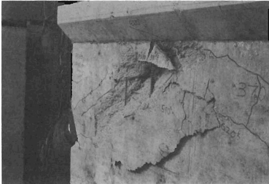
(c) Ultimate load: 590 kips. Side face rupture at point of maximum curvature
