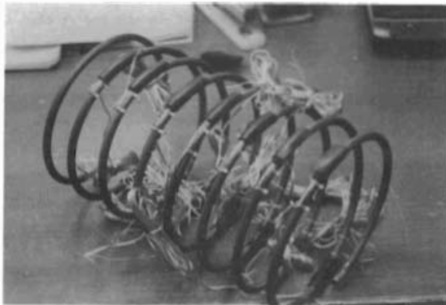
(a) Spirals with strain gages on opposing sides
