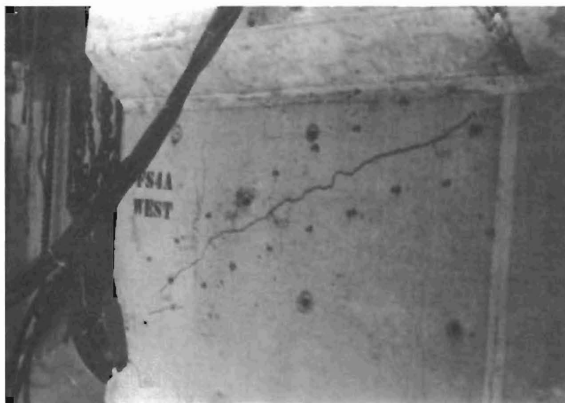
(b) Progression of tendon path crack into anchorage zone with increased load
