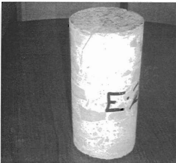
Figure 3.1 Core taken over a surface crack
