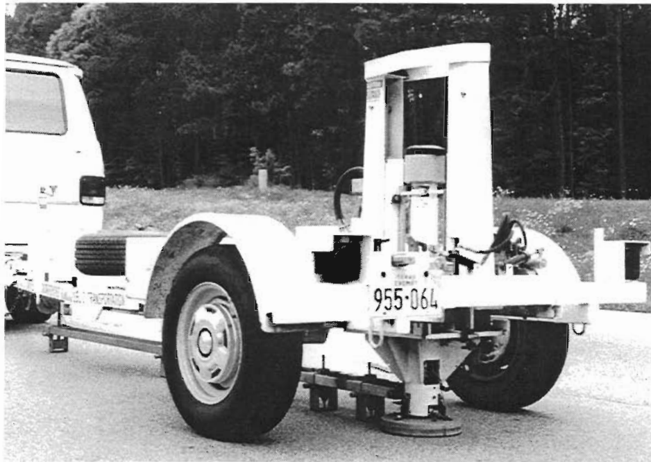
Figure 2.2 Falling weight deflectometer (FWD)
