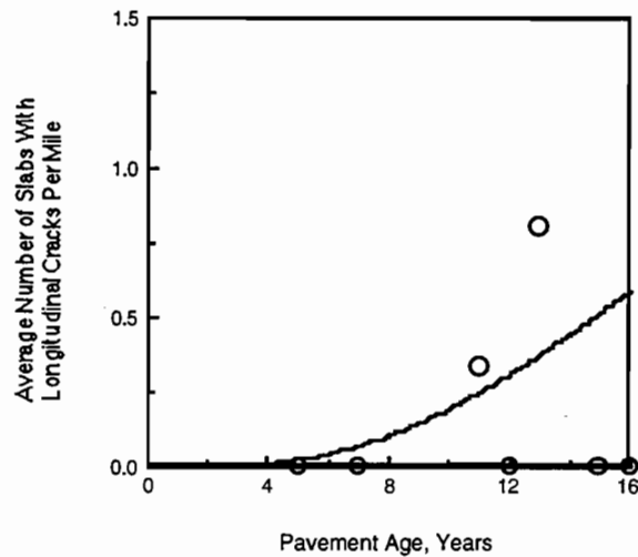
Figure 2.2. Distress prediction model for slabs with longitudinal cracks per mile (1 mile=1.61 km)
