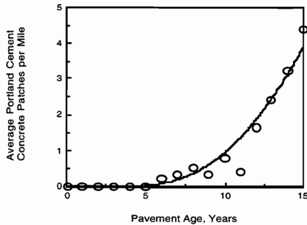
Figure 3.2. Distress prediction model for portland cement concrete patches per mile (1 mile=1.61 km)
