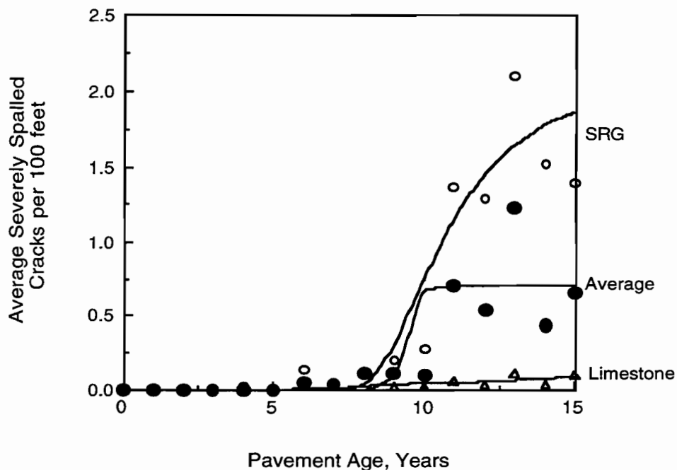
Figure 3.8. Distress prediction models for crack spalling: SRG, LS, and average populations (1 foot=0.304 m)
