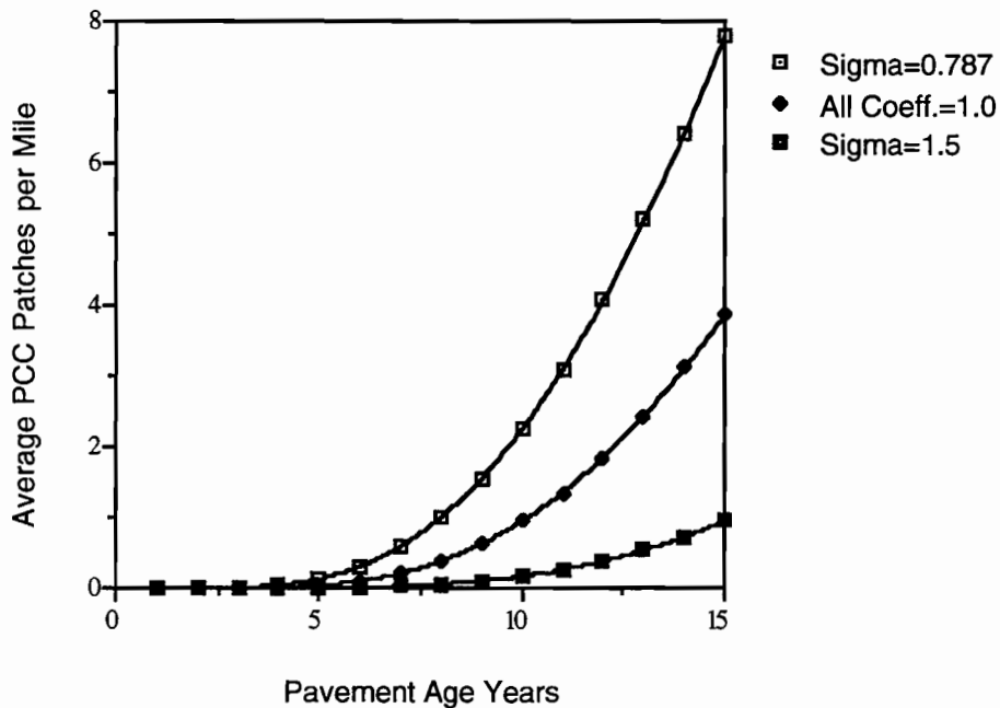
Figure 4.1. Distress curves for PCC patches with and without modifying coefficients (1 mile=1.61 km)
