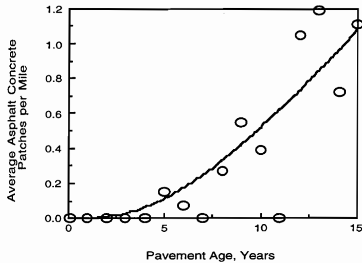
Figure 3.3. Distress prediction model for asphalt concrete patches per mile (1 mile=1.61 km)
