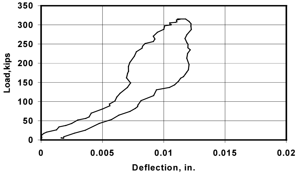
BG3N - North Bearing Pad (East Web)
