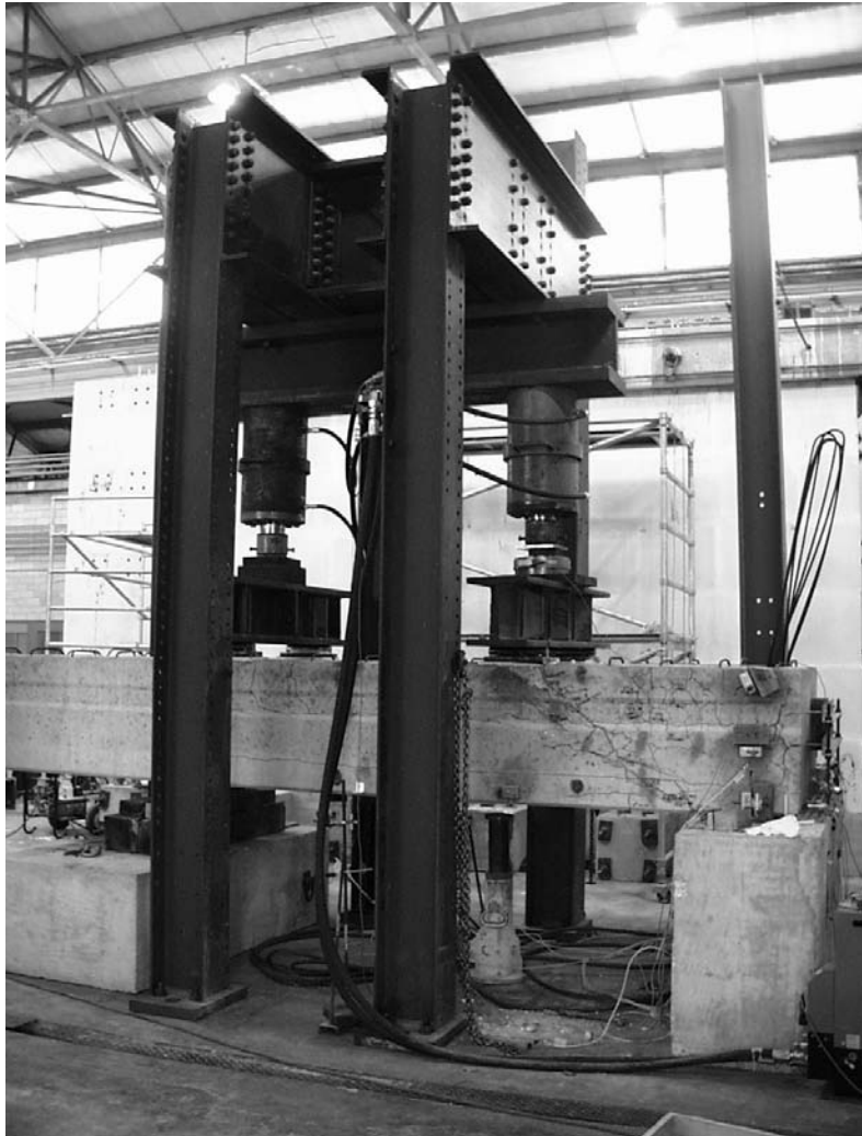
Figure 3.3 Loading setup for shear-dominated fatigue specimens
