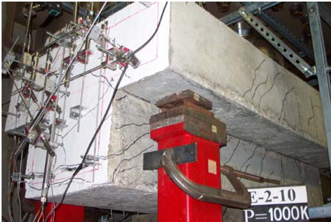
Fig. 3.3(d) Web shear failure in Specimen E-2-10
