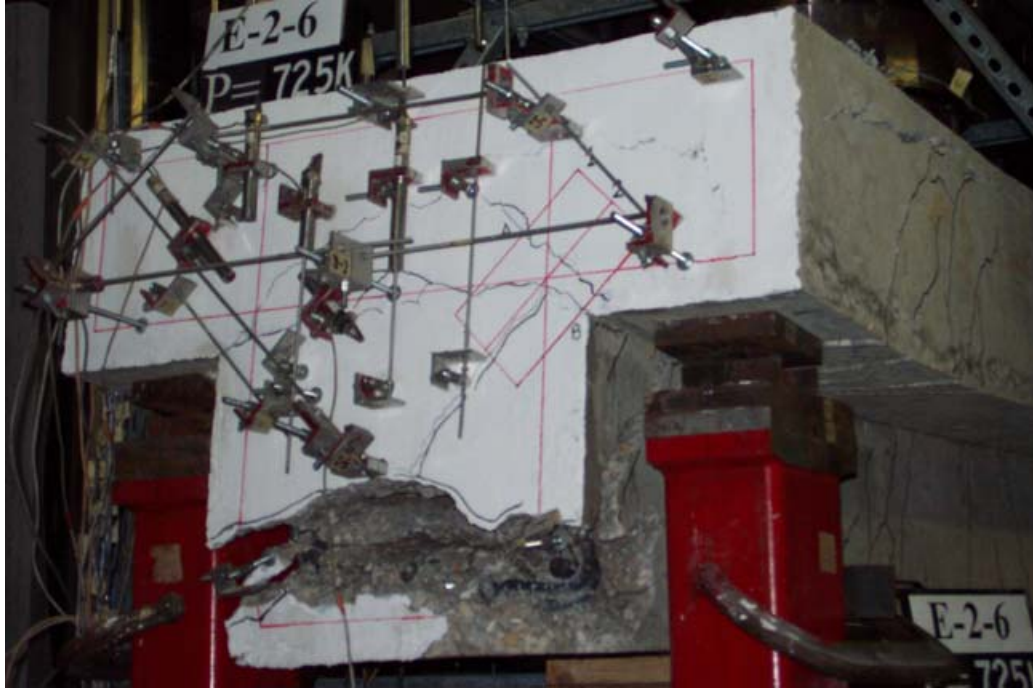
Fig. 3.3(c) Web shear failure in Specimen E-2-6
