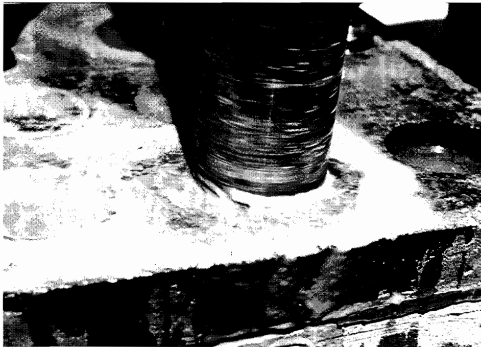
Figure 4.7 Coring a laboratory bond specimen
