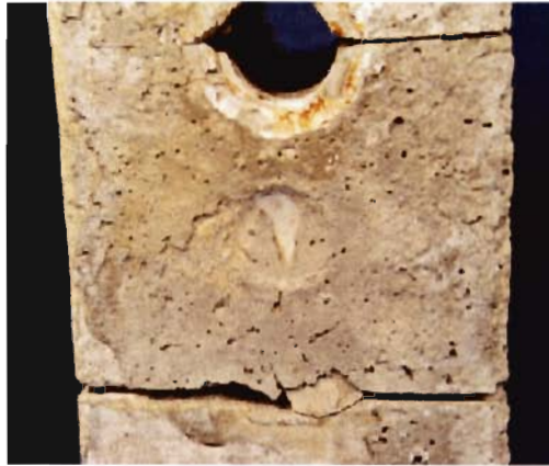
Figure 4.15 – Grout Infiltration Into Joint: Specimen DJ-S-L-CI-1
