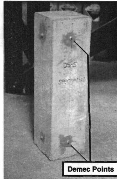
Figure 2.64 Concrete modulus of elasticity test specimen
