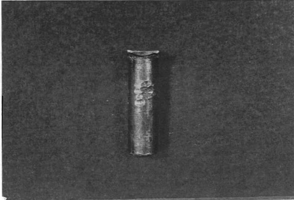
Figure 5-2 Grasping peg showing bearing deformations
