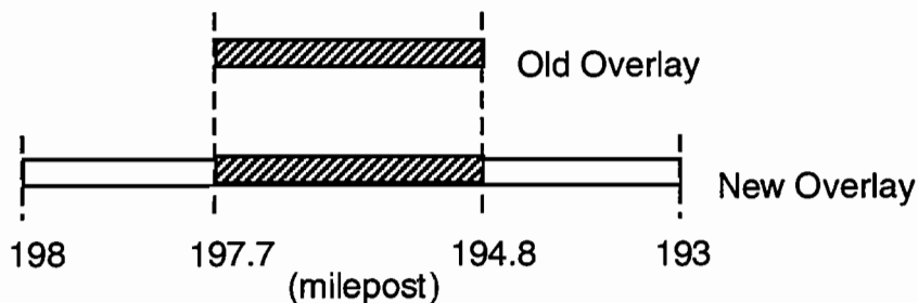
Figure 3.2. Position of old and new overlay profile data
