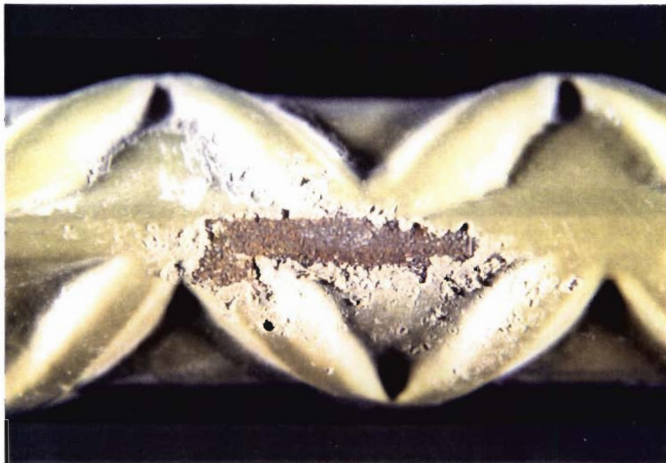
(b) A bar with cross deformations.
