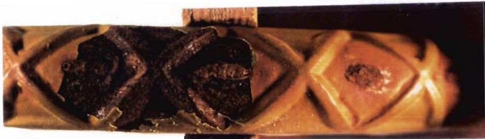
(c) #8 bar with cross deformations
