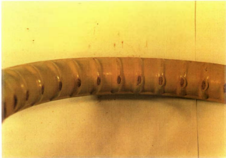
(a) A bar bent at the coating plant
