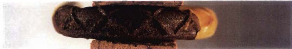
(b) #4 bar with cross deformations
