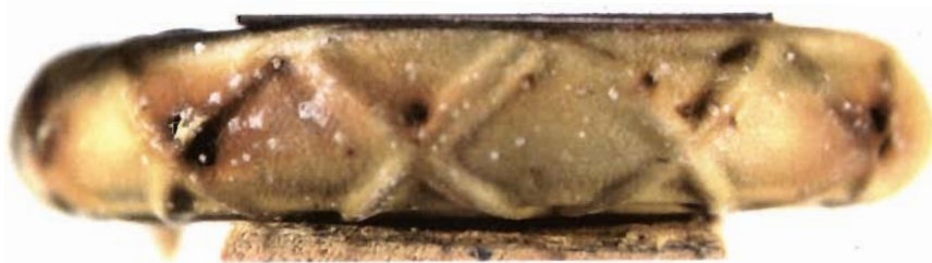
(b) #4 bar with cross deformations (A11 group)
