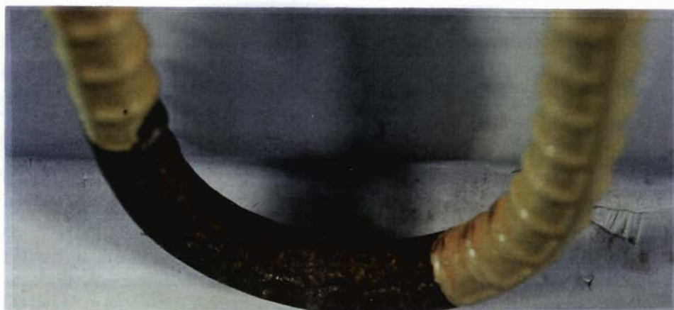
(a) The inside of bend of the bar shown in Figure 3.16(a)
