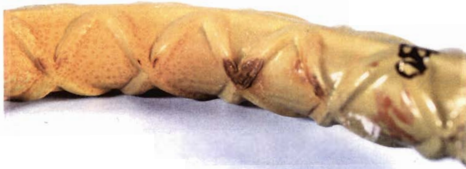
(b) #8 bar with damage area > 2%
