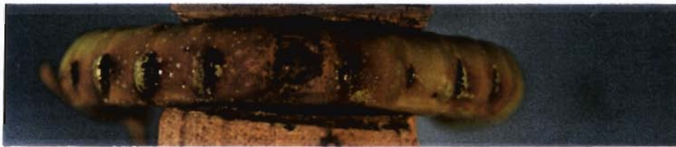
(a) #4 bar with parallel deformations (A3 group)
