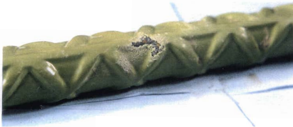
(b) Damage on the side rib
