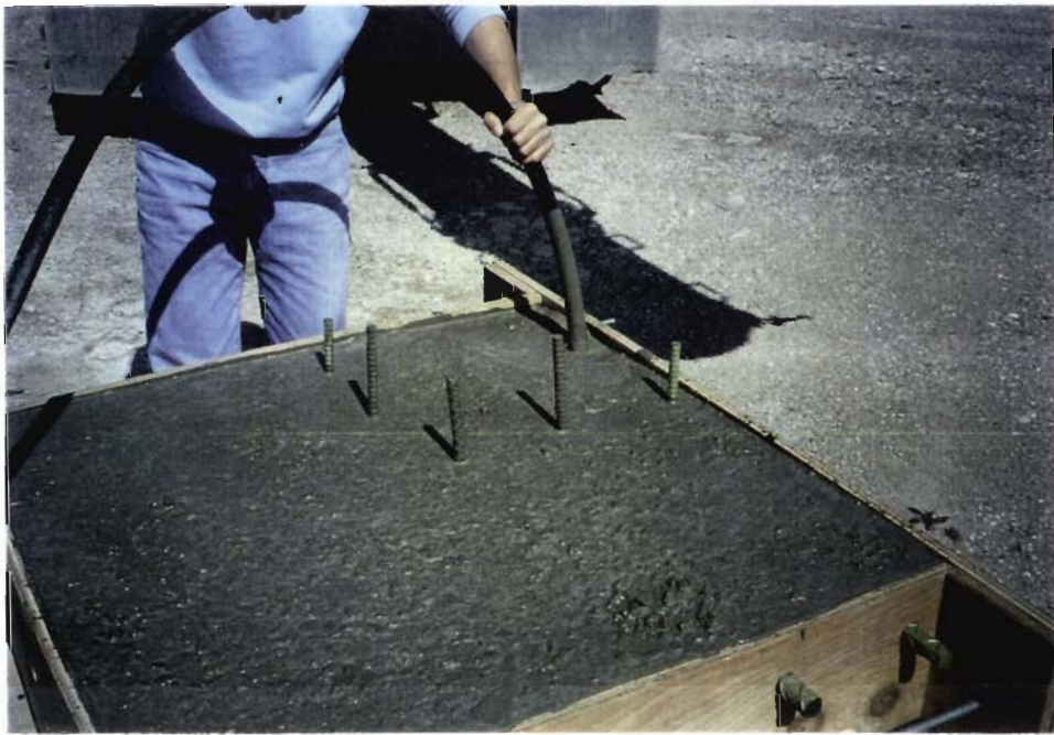
Figure 4.8 Vibration of the column base specimen.
