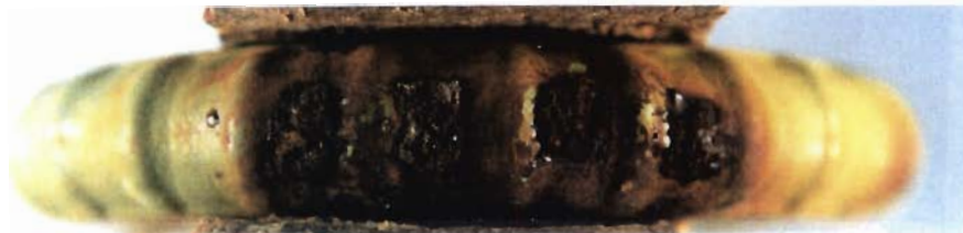
(b) Corrosion in exposed areas
