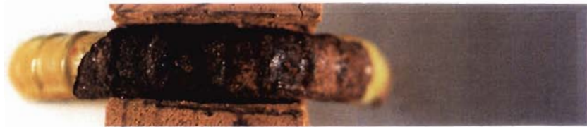
(a) #4 bar with parallel deformations
