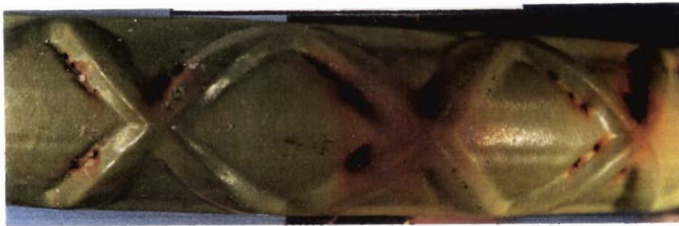
(b) Damage area < 2% (B11 group)
