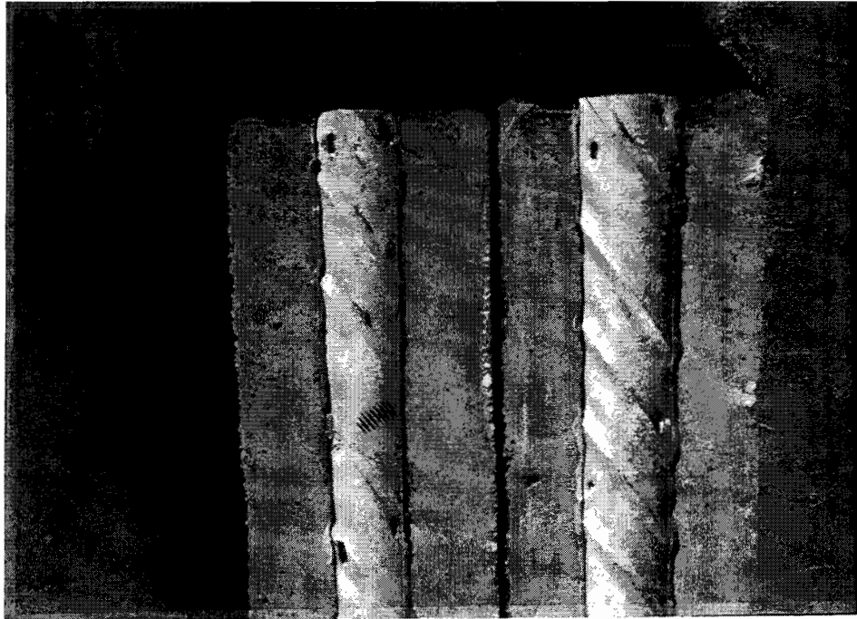
Figure 2.6 Small-scale friction test duct grooving.
