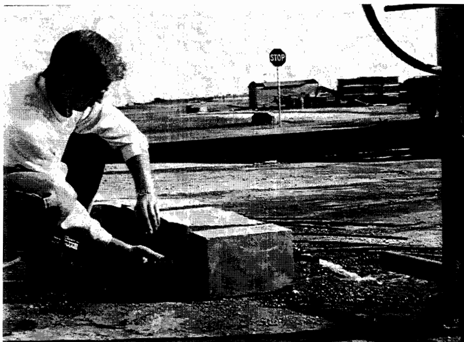
Figure 2.9 Flushing bond test specimen.
