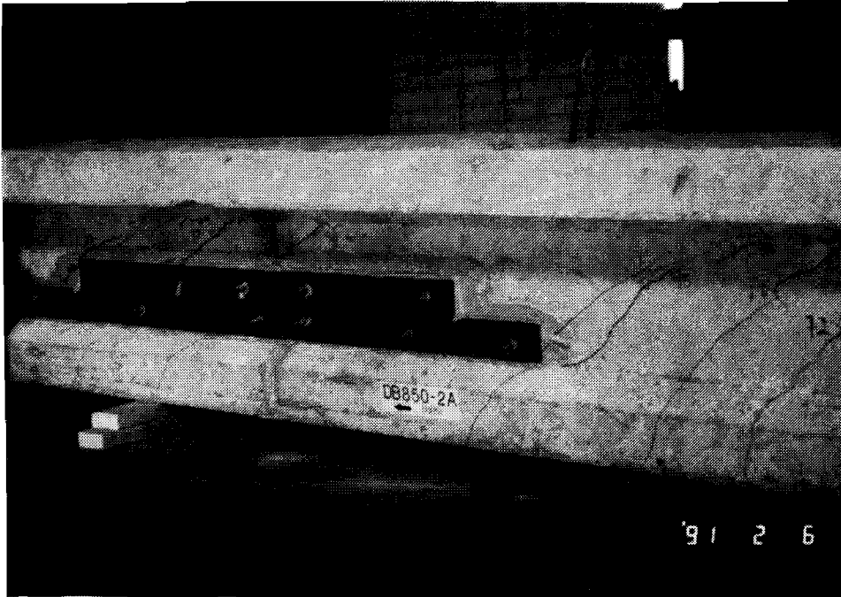
Figure 4.36 Flexural Cracking in the Debond/Transfer Zone, Test DB850-2A (G)
