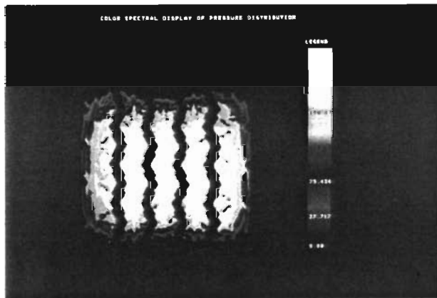
Fig 4.24. Two-dimensional contact pressure plot for the radial Michelin 255/70R/22.5 LR-G tire inflated to 135 psi and loaded to 6,000 pounds.
