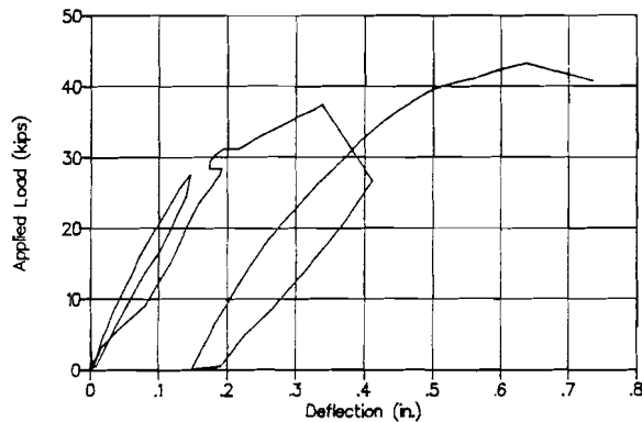
Figure A.1 Applied load vs. load-point deflection for Test 1A-1-0.6.
