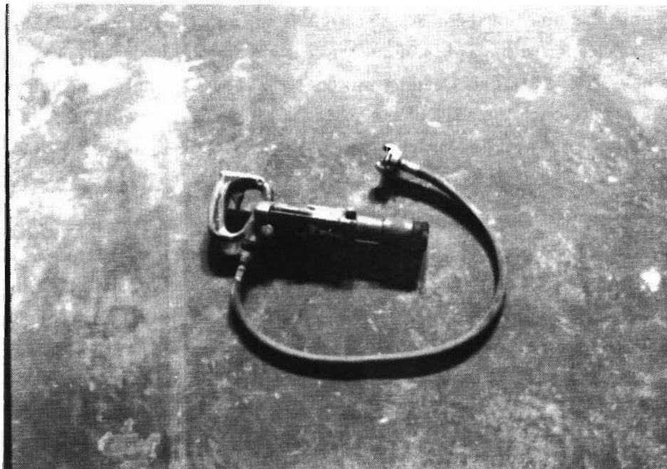
Figure 4.3 Air Drill Used to Drill Holes for Some Adhesive Anchors
