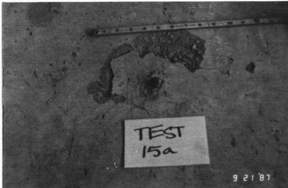
Figure 6.2 Mode 1 Behavior (Shank Fracture, No Slip) for Adhesive and Grouted Anchors
