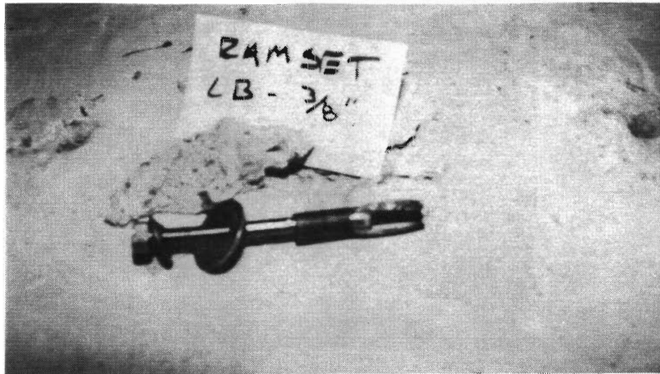
Figure 6.5 Mode 3 Behavior (Pullout Failure) for Expansion and Undercut Anchors
