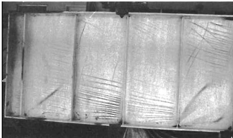
Fig. 3.6 Mode of Failure of \alpha = 0.5 Panel Girder HS-1A, T3
