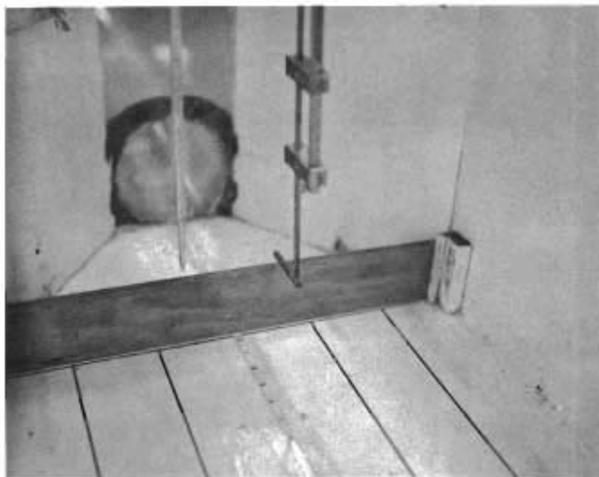
FIGURE 6. PHOTOGRAPH SHOWING POINT GAGE AND PITOT TUBE APPARATUS USED IN EXPERIMENT.
