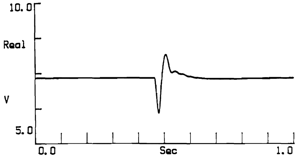
Figure D.33 Raw Displacement Time History of Laser Due to a Half-Sine Pulse Load
