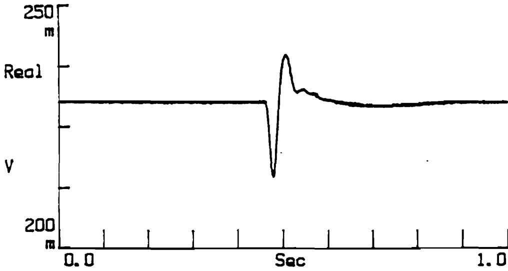
Figure D.29 Raw Displacement Time History of Proximeter Due to a Half-Sine Pulse Load
