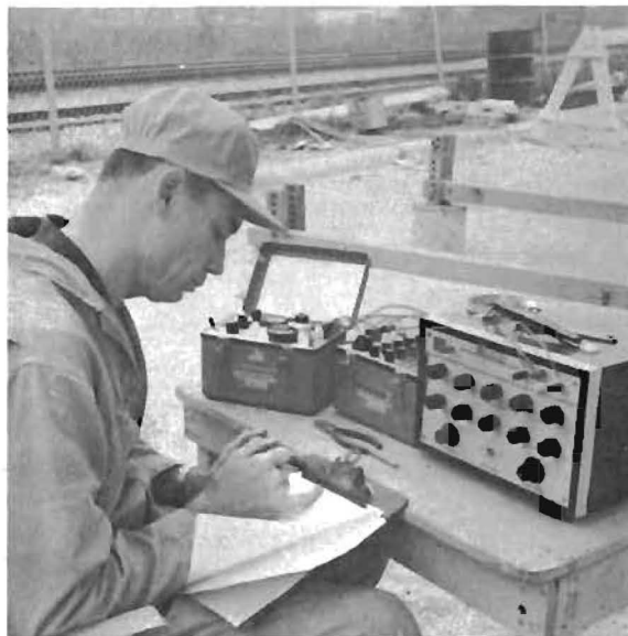
Fig. 5.14. Taking Mustran Cell Test Data Utilizing Strain Indicator in Conjunction with Two Switch and Balance Units
