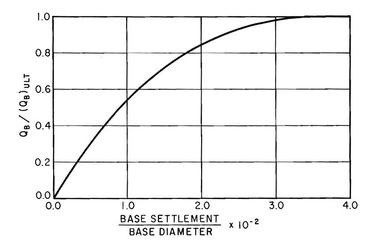
Fig. 13.2. Design Curve for Base Load Versus Settlement for Drilled Shafts in Beaumont Clay
