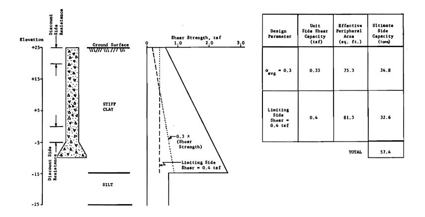
Fig. 13.4. Side Capacity for Design Example Problem No. 2
