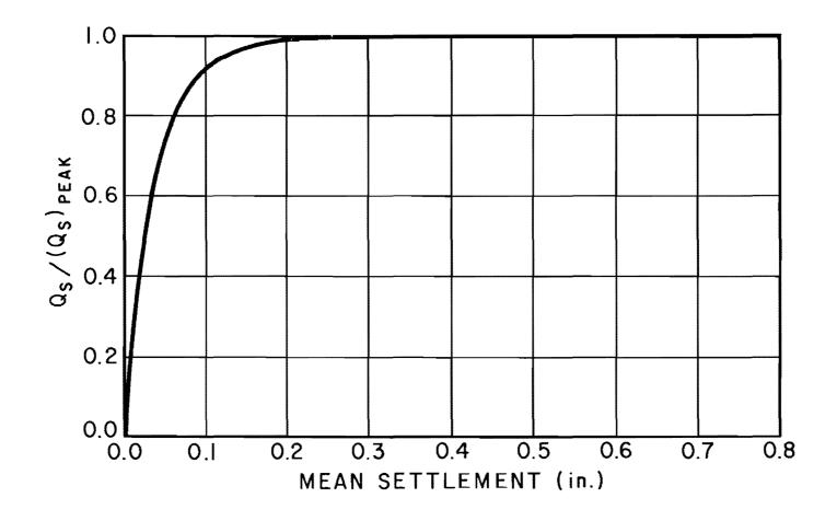
Fig. 13.1. Design Curve for Side Load Versus Settlement for Drilled Shafts in Beaumont Clay
