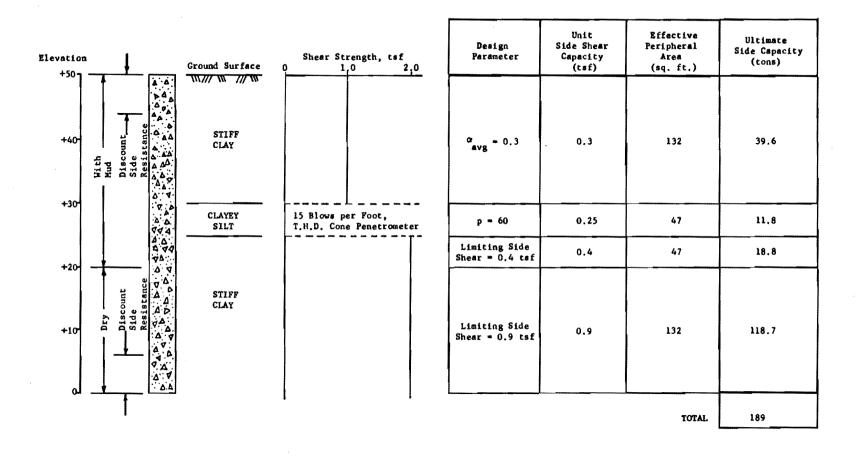
Fig. 13.3. Side Capacity for Design Example Problem No. 1
