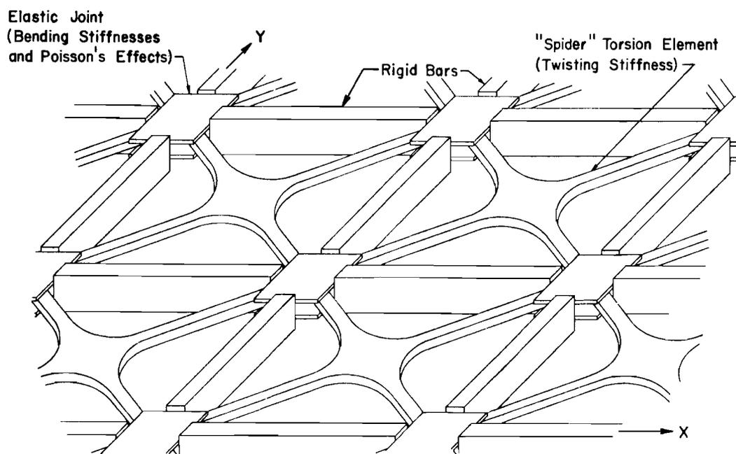
Fig 19. Discrete-element model of slab or plate.
