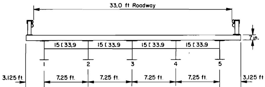
Fig 26. Three-span highway bridge.
