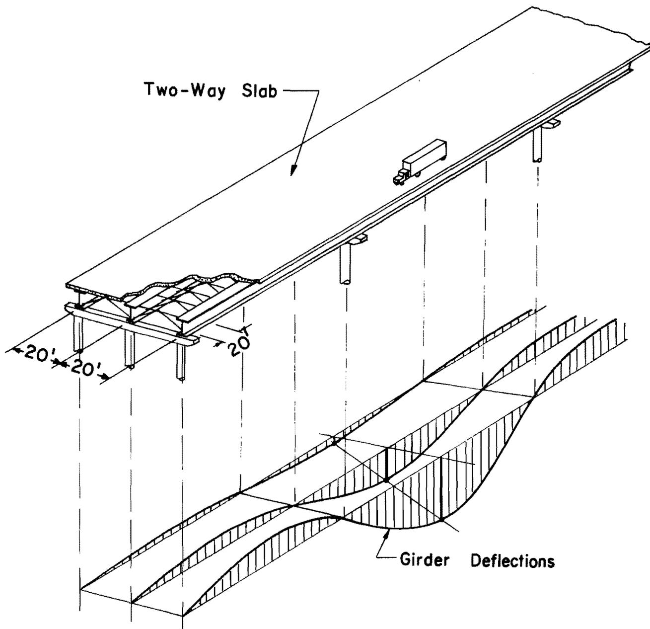
Fig 18. A typical bridge floor system.
