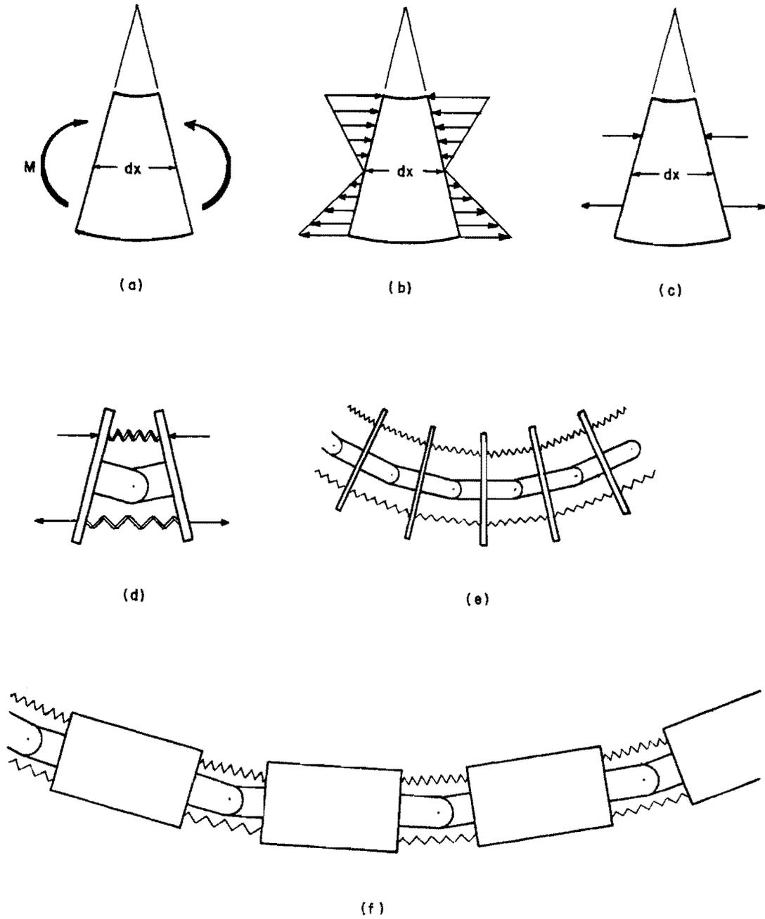
Fig 1. Mechanical representation of a conventional beam.
