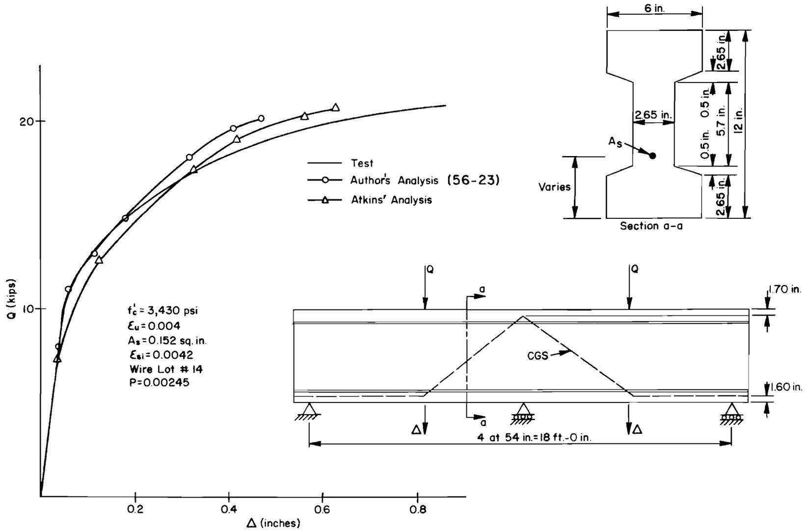
Fig 9. Two-span prestressed beam tested at the University of Illinois.
