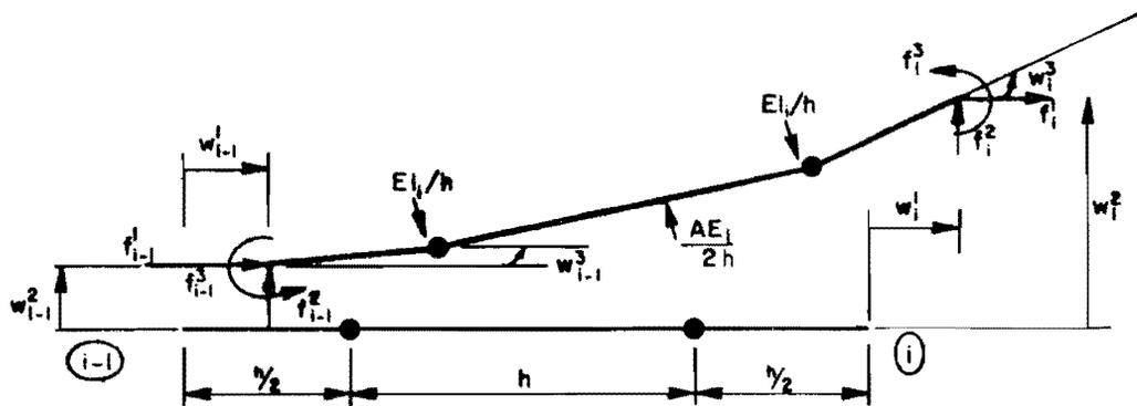
(b) Discrete-line-element model of element  $i$ .
