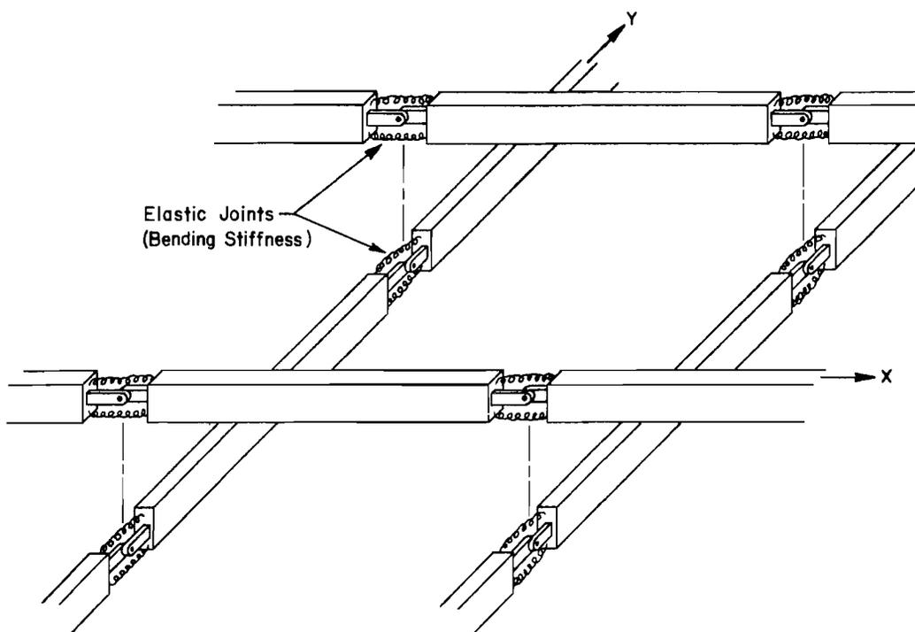
Fig 20. Discrete-element model of grid system.
