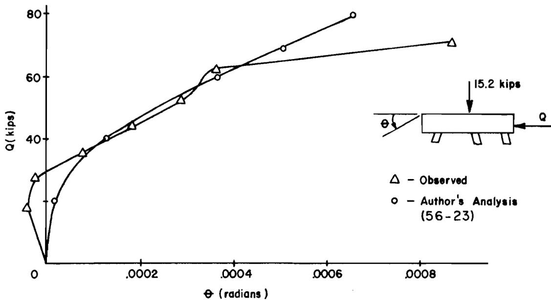
Fig 11. Load-displacement and load-rotation responses for three-pile bent.
