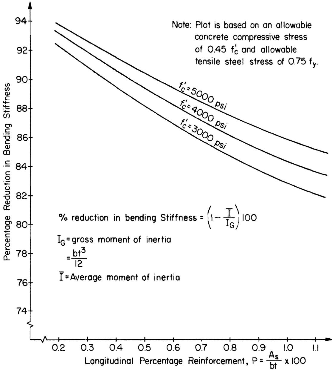
Fig 25. Reduction in bending stiffness at cracks.
