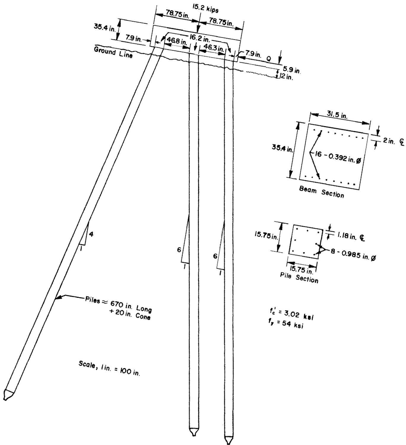
Fig 10. Soil-supported bent tested at Galati, Rumania.
