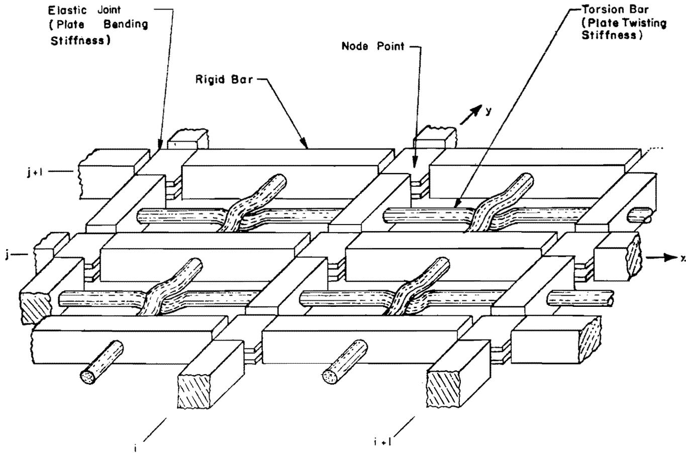
Fig 13. Discrete-element model of a plate or slab.
