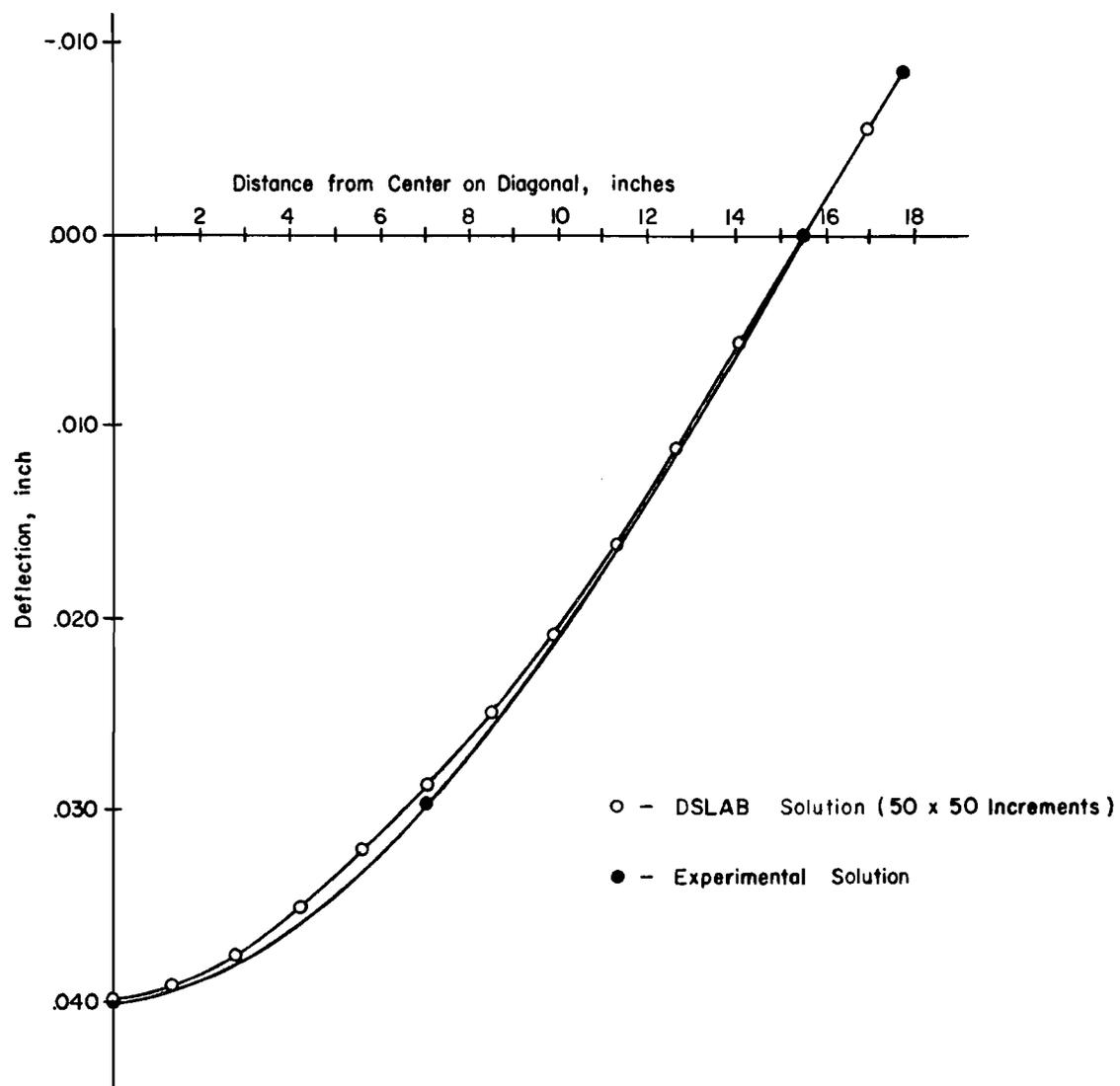
Fig 24. Experimental and analytical deflections.
