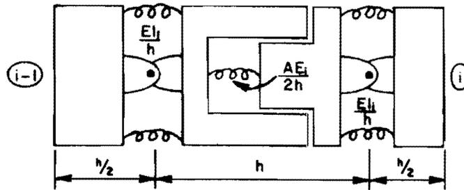
(a) Mechanical model of element  $i$ .
