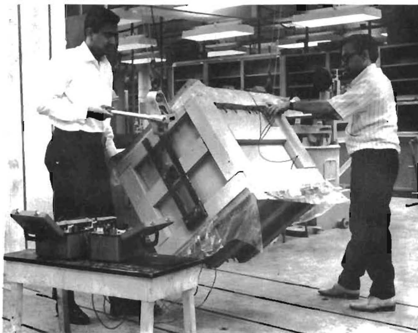
Fig 34. Method of overturning the box.
