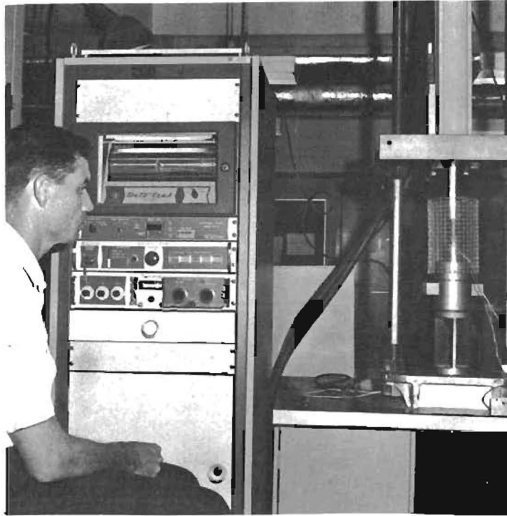
Fig 2.6. Load cell calibration; loading control.
