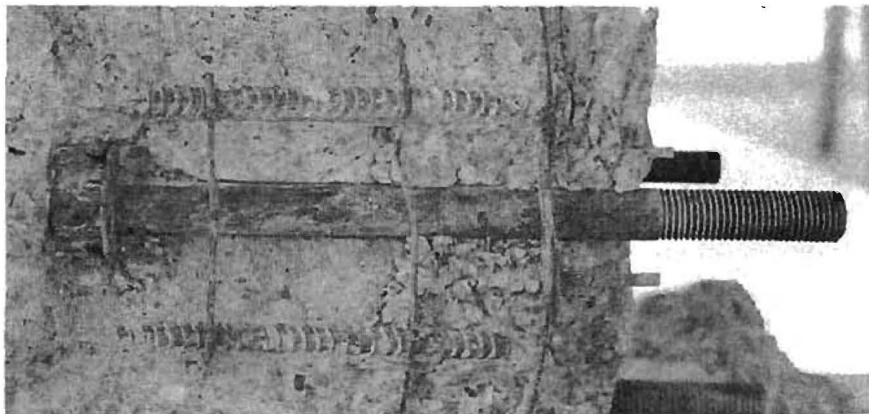
Fig. 23. Movement and distortion of nut and washer
