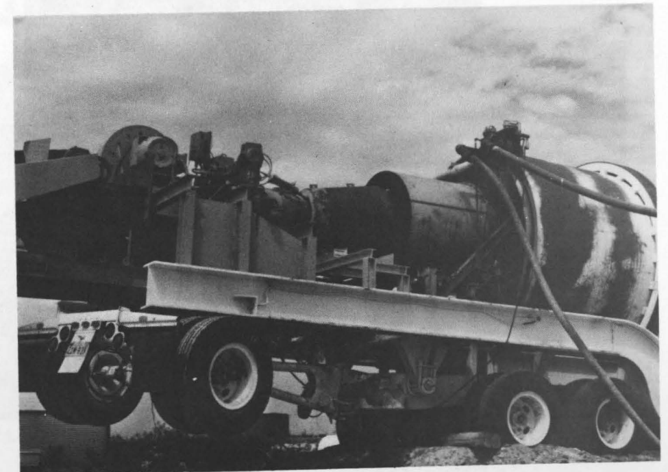
Picture #6 - Feed-belt inducing materials into bottom of drum beneath flame.
