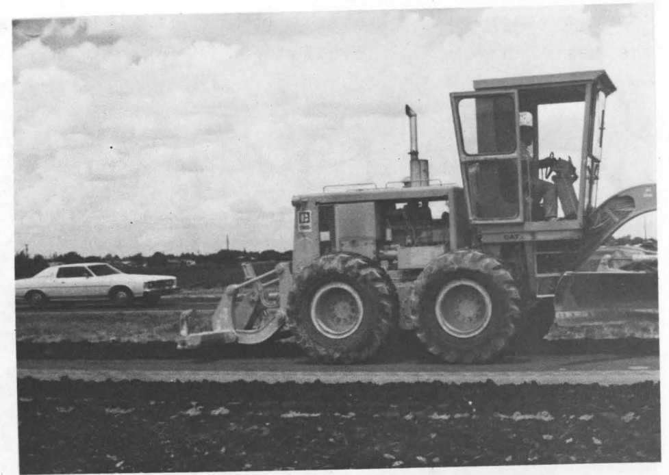
Picture #1 - Ripper teeth mounted on the rear of a D-14 motor grader.
