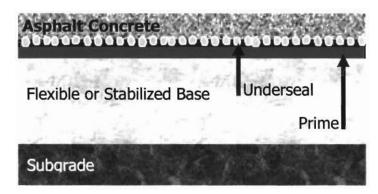
Figure 2 Schematic of a Pavement with Surface Treatment as Underseal
