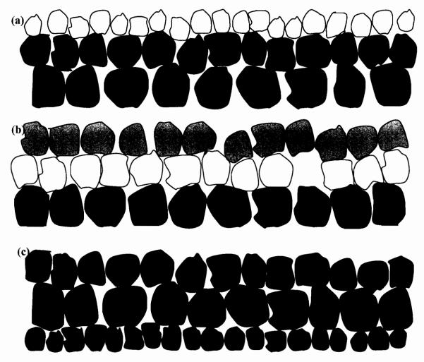
Figure 10. Aggregate Grade Combinations Used in 3-CST (a) Grade 5 on Grade 4 on Grade 3 (b) Grade 4 on Grade 4 on Grade 3 (c) Grade 4 on Grade 5.
