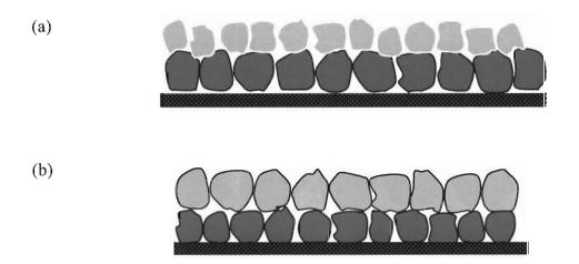
**Figure 9** Aggregate Grade Combinations Used in 2-CST (a) Grade 4 on Grade 3 (b) Grade 3 on Grade 4
