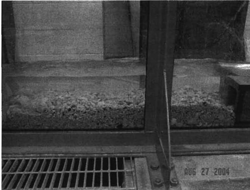
Figure 8. Upstream portion of model looking towards culvert. Entire "road bed" is submerged.
