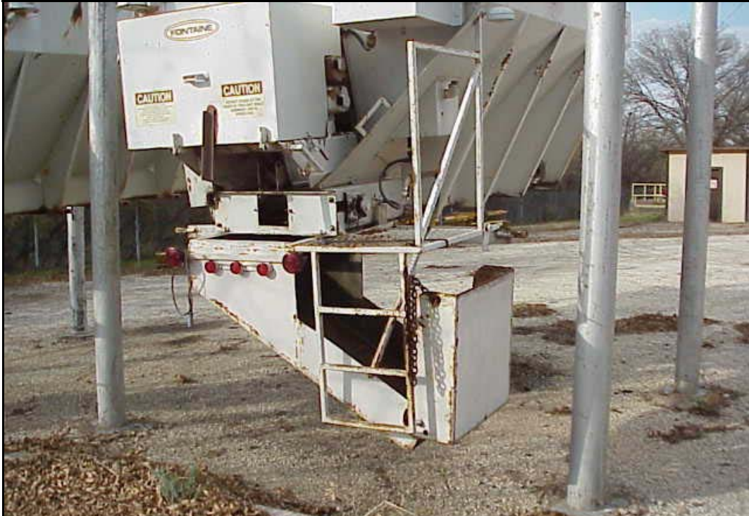
FIG. 7.18 Modified V-Box Side Discharge Spreader: Side View, San Angelo District (see San Angelo District Profile, Photo 17)
