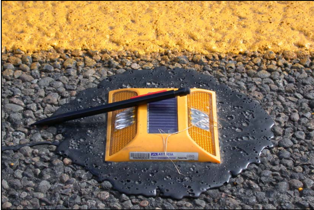
FIG 5.19 Experimental High-Visibility RPM with Photoelectric Cell that Lights up During Rainfall Events, Atlanta District (see Atlanta District Profile, Photo 31)
