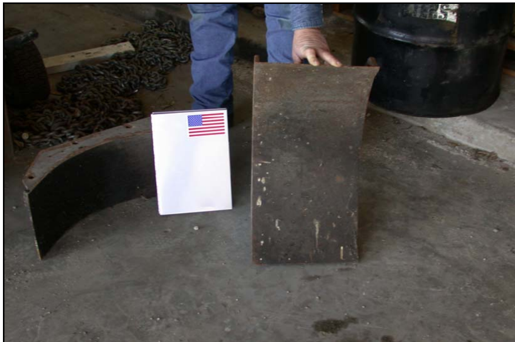
FIG. 7.5 Curved Shoe for Midland Machinery Road Widener, Fort Worth District (see Fort Worth District Profile, Photo 29)
