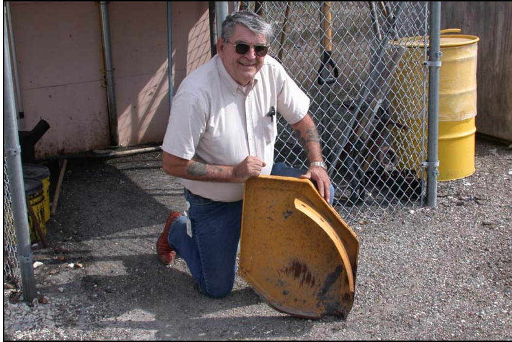
FIG. 7.3 Motor Grader Blade Shoe for Pulling Shoulders, Corpus Christi District (see Corpus Christi District Profile, Photo 9)
