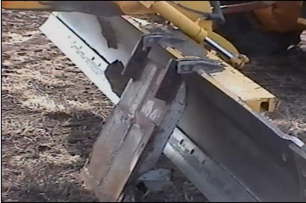
FIG. 7.4 Motor Grader Blade Shoe for Road Widening, Amarillo District
