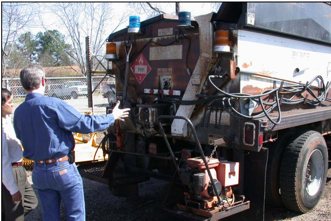
FIG. 7.27 Pro-Patch TCM 415-60 Pothole Repair Truck, Tyler District (see Tyler District Profile, Photo 15)
